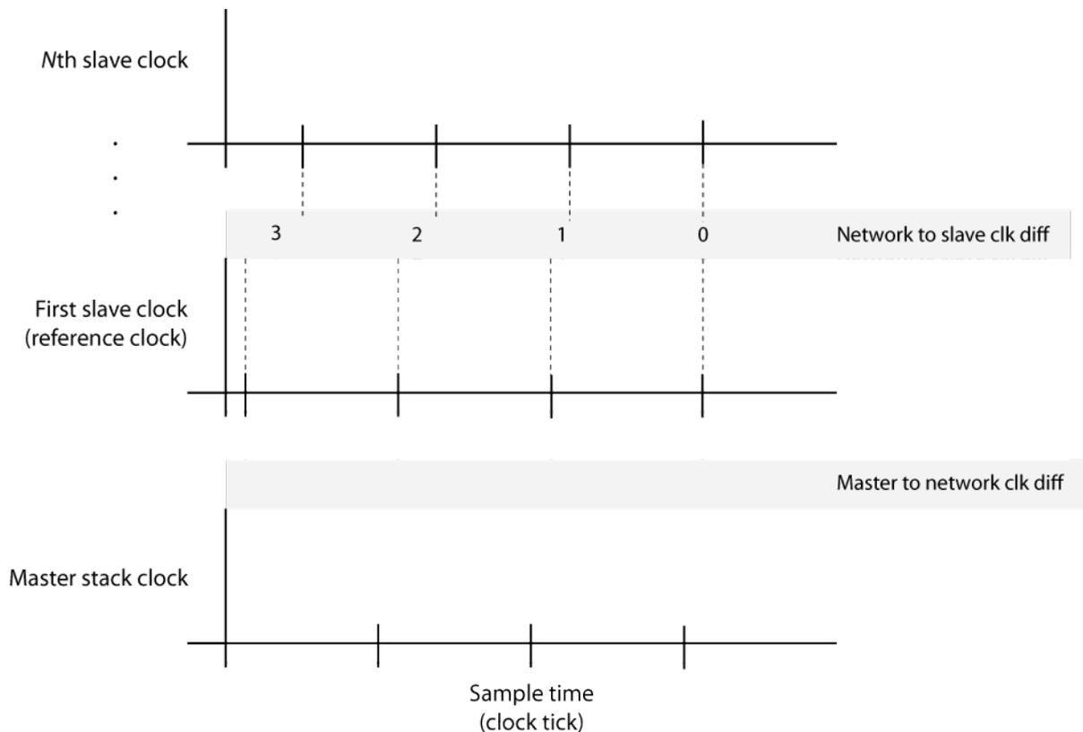
In phase 2, the algorithm shifts the sample time of the master stack running on the target computer to align with the first slave node clock. In that process, the EtherCAT Init block output value `MasterToNetworkClkDiff` decreases to near zero.
