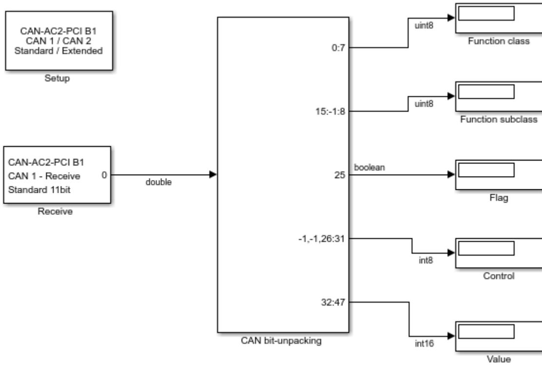
Often it makes sense to test the bit-packing and unpacking operations in a Simulink model (simulation) before building the real-time application. Both blocks work the same way either in the Simulink system or the generated code. By combining the two models shown so far, a third model emerges that can be used to simulate the behavior.
