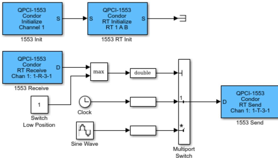
The QPCI-1553 RT Initialize block configures the board for Remote Terminal operation on channel 1 of the board. The QPCI-1553 RT Initialize block configures the Remote Terminal 1 to monitor buses A and B for incoming messages and configure the active transmit and receive sub addresses. The QPCI-1553 Receive and Send blocks use sub address 3 for both transmit and receive. Note the message parameters notation 1-R-3-1 on the QPCI-1553 Receive and Send blocks. This notation has the format:
