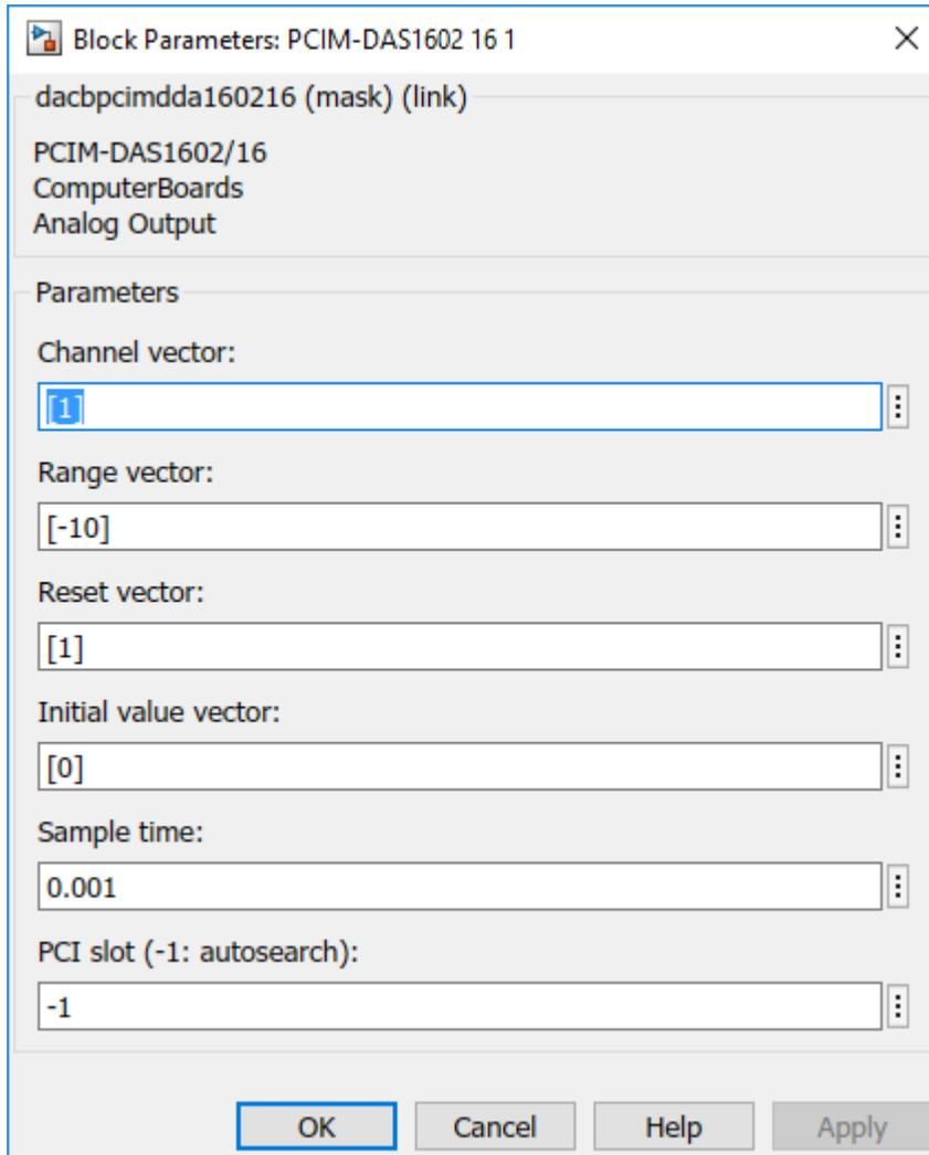
If you change the target object property `SampleTime`, the sample times you entered in both of the I/O blocks are set to the new value. The step size you entered in the Configuration Parameters dialog box remains unchanged.
