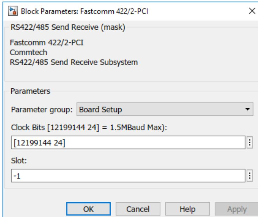
After you define a maximum baud, to set a unique baud for each channel, specify a different baud divisor for each channel. For example, you can set Channel 1 to a baud of 750000 (1500000/2) and Channel 2 to a baud of 1500000 (1500000/1). To set Channel 1 to a baud of 750000, with the Fastcom 422/2-PCI Send Receive block with the **Parameter group** parameter set to `Basic Setup`, set
