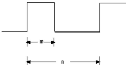
For a base frequency  $b$ , this algorithm results in a rectangular output signal of frequency  $b/n$  and duty cycle  $m/n$ . Because  $m$  and  $n$  must be integers, it is not possible to provide a continuous range of output frequencies and duty cycles with perfect exactness.
