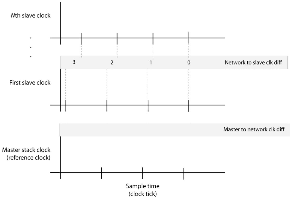
In phase 2, the algorithm shifts the sample time of the first DC-enabled slave node to align with the clock of the master stack. In that process, the value `MasterToNetworkClkDiff` decreases to near zero. The algorithm shifts the sample time of the other network nodes to stay aligned with the first slave node clock. In that process, the value of `NetworkToSlaveClkDiff` first increases, then decreases to near zero.
