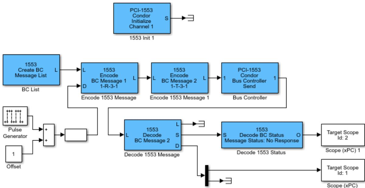
The PCI-1553 Initialize block configures a Bus Controller on channel 1 of the board. This block also tells the board to reserve five message buffers. This number must be at least as large as the longest list of messages that you send.
