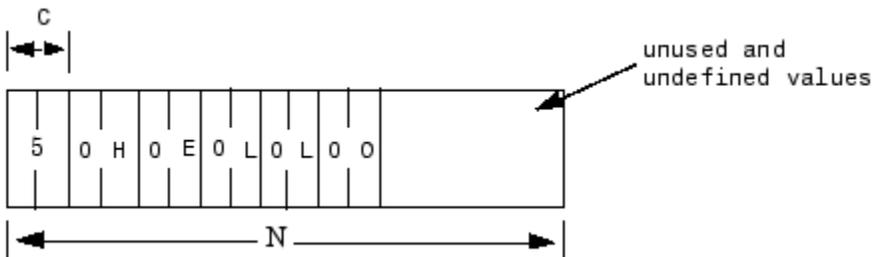
These serial blocks interpret each entry in the vector as a single character. The low-level Send block writes the low-order byte of each entry to the UART. The 16-bit and 32-bit data types allow the embedding of 8-bit data values, including 0. The 8-bit data type is most useful with the ASCII Encode and Decode blocks. The 16-bit and 32-bit data types are most useful for binary data streams.
