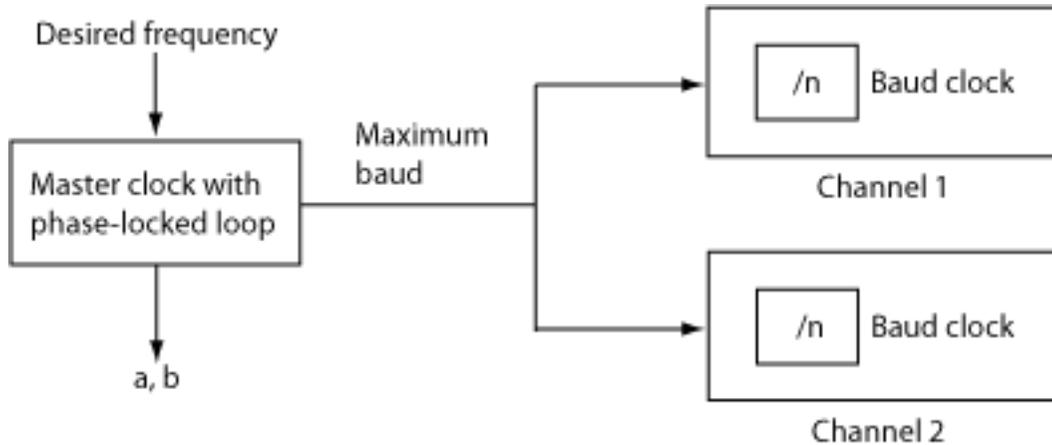
To set the block parameters for this board, calculate a maximum baud, as follows. This procedure assumes that both channels require different baud. Determine a common base clock that can be divided to produce the required baud for both channels, as follows:
