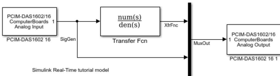
You cannot run this model unless the required I/O board is installed in your target computer. However, you can substitute driver blocks for another I/O board that is installed in the target computer.
